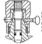
Finger screw Option (Code "F") provides this thumbscrew in place of set screw.
