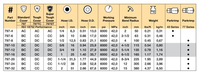
Application: Petroleum-based hydraulic fluids, lubricating oils
