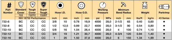
Application: Petroleum base hydraulic fluids and lubricating oils
